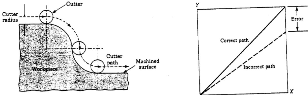
(a) Continuous path cutting and (b) Position error caused by the velocity error
