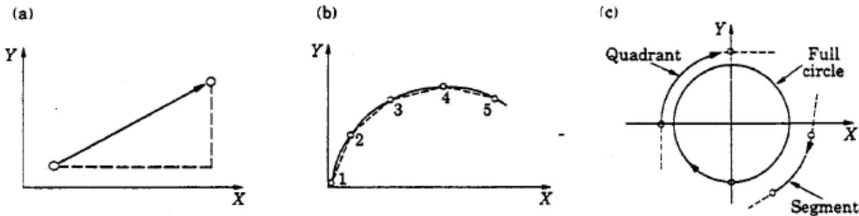
Types of interpolation (a) linear, (b) continuous path approximated by incremental straight lines, and (c) circular
