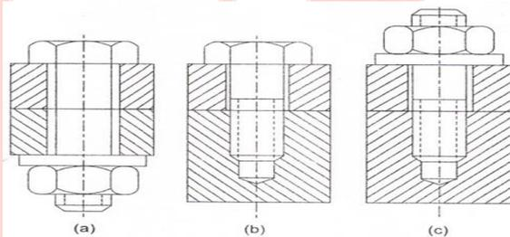
Types of Screw Fastening: (a) Through Bolt (b) Tap Bolt (c) Stud
