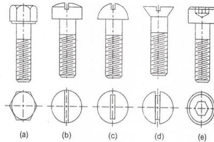
Cap Screws with Different Heads: (a) Hexagonal (b) Filister (c) Button (d) Flat (e) Hexagonal S
